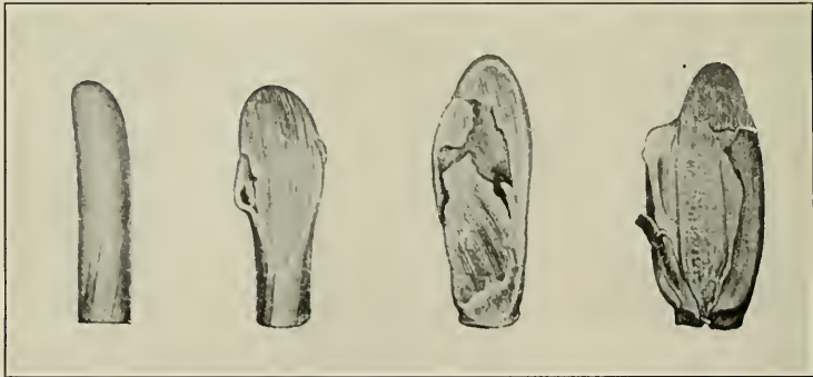
Fig. 587.—Four common types of lateral Mauser ricochet bullets (from Makins' "Surgical Experiences," etc.).
